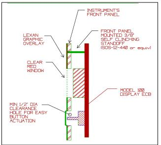
Figure 5: Typical Front Panel Installation
