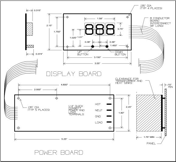
Figure 4: Mechanical Mounting Dimensions
