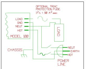
Figure 2: Typical Load Connection
